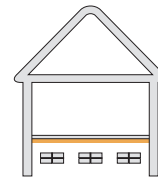
Sub-floor solid perimeter
