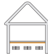
Sub-floor solid perimeter
