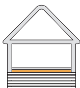
Sub-floor with timber battens
